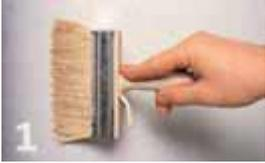
The surface must be consistent, flat and clean. It must be dry and free of grease like substances. If the surface is porous then apply a layer of bonding primer. Allow to dry for at least two hours and then you can begin.
